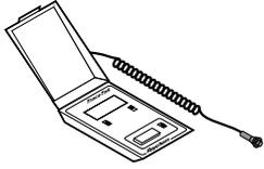
Portable Test Box. Battery operated device for testing TraceTek sensing cables. Allows testing of an individual length or up to 2000ft (1000 m) of sensing cable. Useful for installation and maintenance of extensive systems. TT-PTB-1000 has plastic socket connector on flexible cord. Test box kit includes adaptors (plastic-to-metal and plastic-to-alligator clip) along with modular end terminations. Part number is 486437-000.
