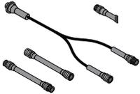
Optional kit useful for testing systems with metal connectors. Includes several adaptors with metal connectors: Y adaptor with both pin and socket, socket-to-socket adaptor, pin-to-pin adaptor and end termination with socket adaptor. Part number is 646003-000.
